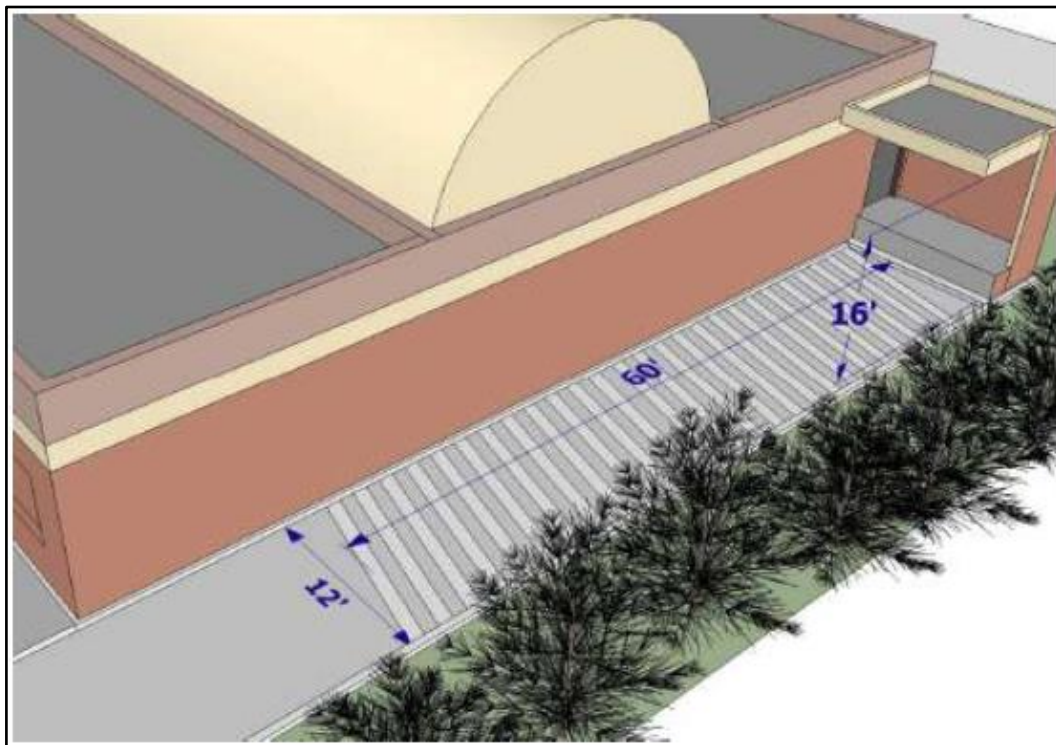
Figure 6-10: OFF-STREET LOADING REQUIREMENTS
